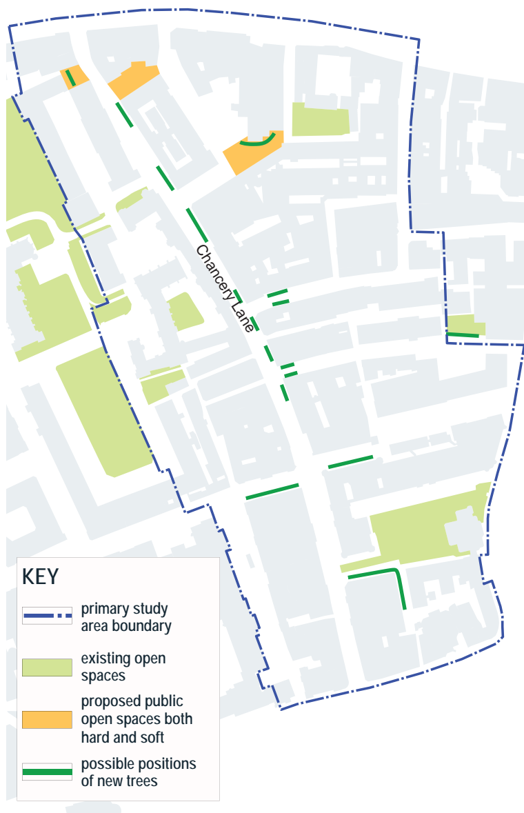
Strategy diagram showing proposed sites for new open space and tree planting
